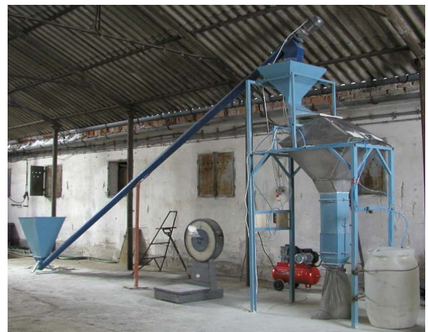
Photo 5: Gravitational Zeolite Dust Modifying Equipment
