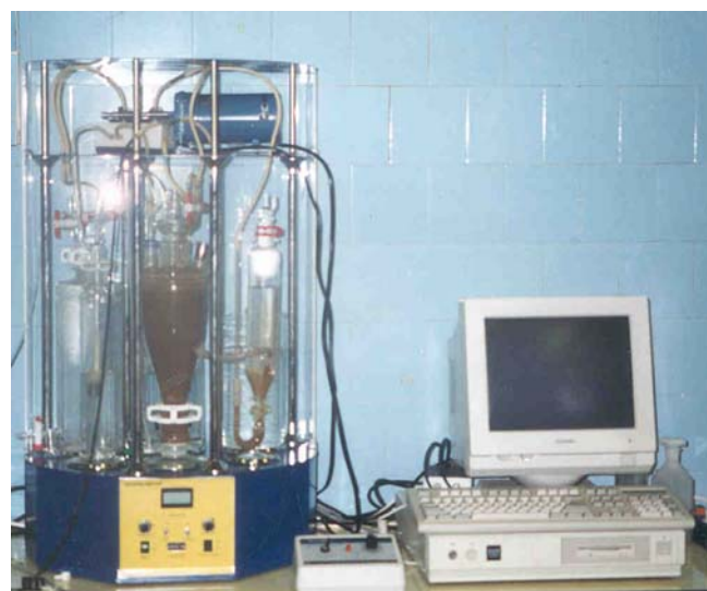
Photo 1 Picture of lab-scale wastewater treatment plant
